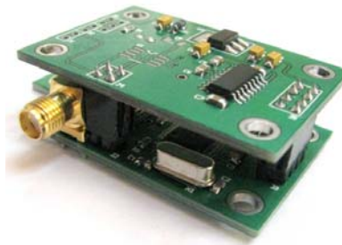
Figure 2: ARN-SGPS-Bxx electronic board with RS232 or RS485 output
