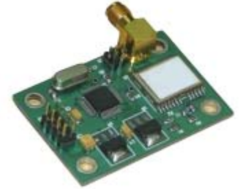
Figure 3: ARN-SGPS-Bxx electronic board with TTL output
